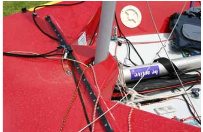
Very neat foredeck arrangement on Boobs 'R Us including mast gate and boom vang attachment point. The mast is from Carbon Concepts in Melbourne.
