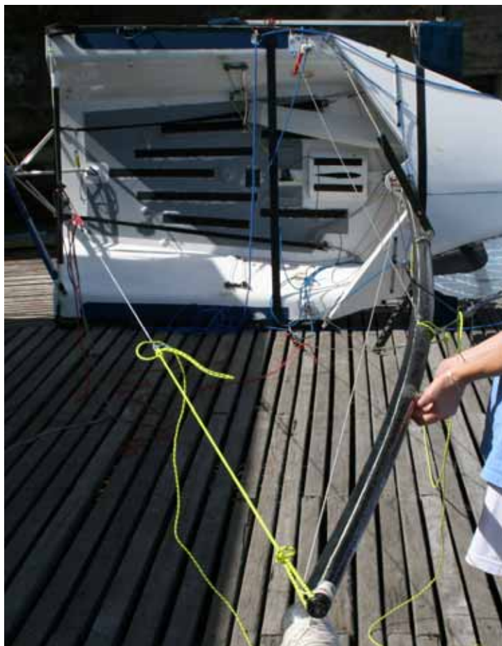
Above: Typically the luff round needed for a mainsail can be measured by loading the mast to a pre-determined load, and then measuring the resulting deflection of the mast from a string line running from the tip to the gooseneck.
