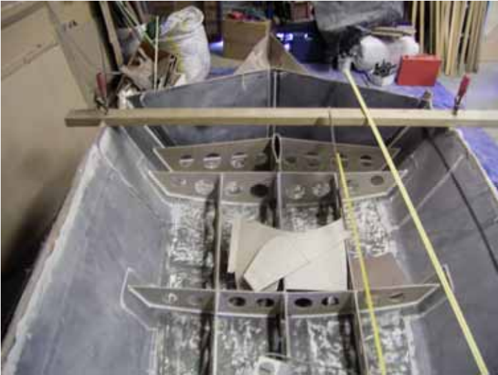
Above: Frames and the bulkheads bonded in place on Wayne Torpy's rebuild of Rope City 3055 .
