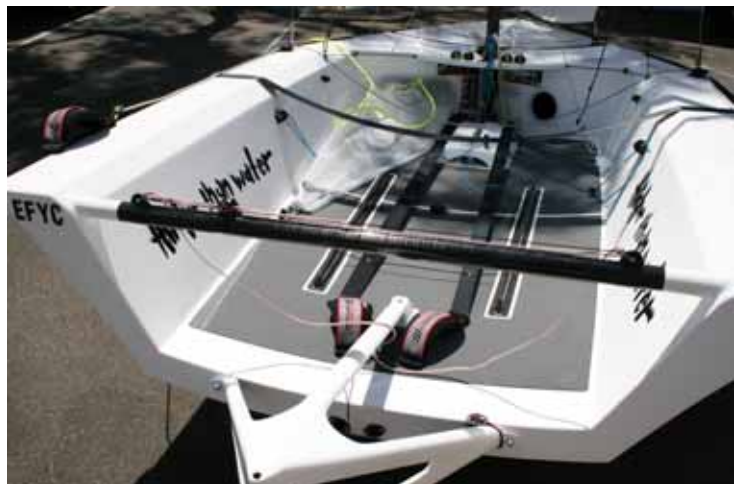
Above: A top line modern Cherub will typically be equipped with all carbon spars, a self tacker for the jib, a carbon or stainless steel tube rudder gantry and foils with a very high quality finish.
