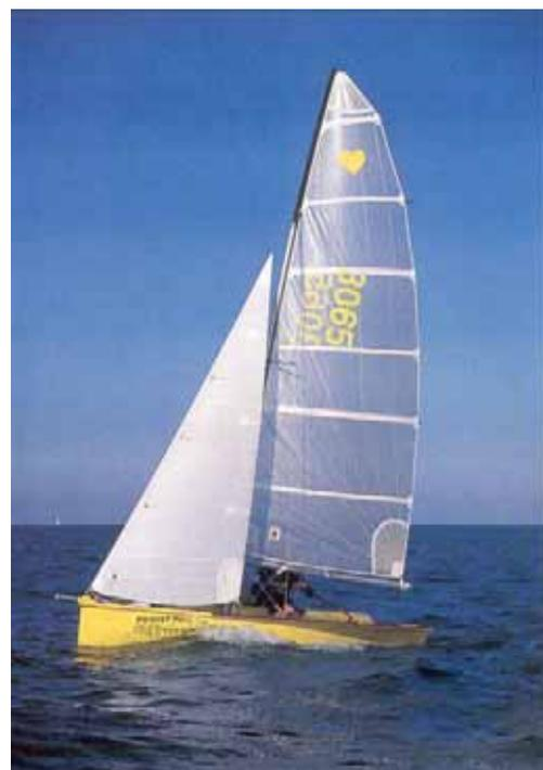
*Working sail plan is unchanged; asymmetric measures 15.5sq m.*
