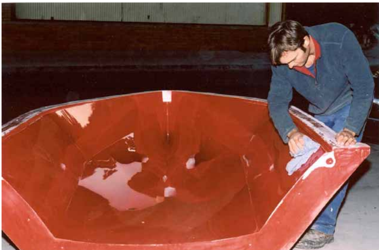
The Matthews Cherub mould features straight lines aft and is narrow on the waterline at the transom. (Rolf Lunsmann photo)
