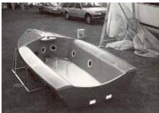
*The production hull has mouldings for mast gate, spinnaker chute and centreboard case.*
